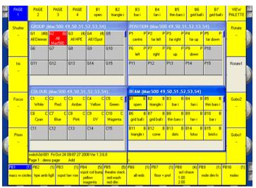
The MagicQ desk uses a **colour touchscreen** with additional hardware buttons, patched to contextual **softbutton control**. The MagicQ PC screen replicates the touchscreen minus the hard buttons round the screen area. The large yellow squares around the edge provide softbuttons that change as you enter different screens. The screen layouts are customisable and provide the **flexible interface** for the console.
