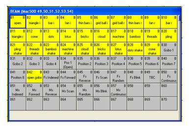
The MagicQ often displays selection grids on it's **main screen**. These squares are softbuttons that hold the button label and can be used for selection. The grids display Fixtures, Groups, Palettes and other selectable stuff. Using MagicQ PC without a touchscreen, the mouse is used to click on the square.
